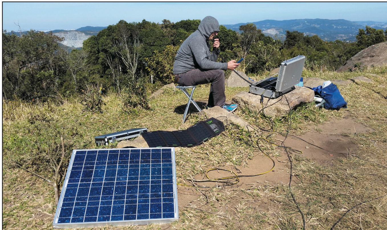
Here's PY2CDR operating. The station consists of: FT-817ND, MOXON 6 meter, DK7ZB Light 6-element 2 meter, 60-watt solar panel 12 volts, 18-watt solar panel 5 volts, and 18-Ah batteries.
